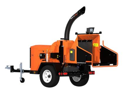
The <u>Crary Bear Cat CH611DH towable</u> Chipper is powered by a reliable Kubota diesel engine with 24.8 gross horsepower. The 165 lb. cantilevered rotor is equipped with four reversible heat-treated blades and eats through branches quickly. The four-sided anvil is adjustable to ensure you get the best chip possible.
