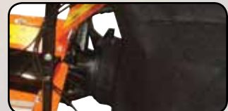
A slotted mechanism keeps the bag securely attached to the vac's body
