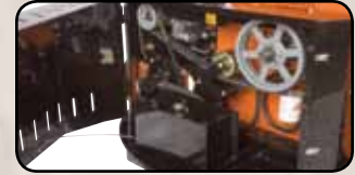
Hinged cover allows easy access to belt drives for in-field servicing
