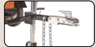
2" ball coupler with safety chains and stabilizer jack are standard
