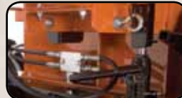
Hydraulic jack easily raises and lowers the feed roller for easy in-field servicing
