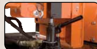
Hydraulic jack easily raises and lowers the feed roller for easy in-field servicing
