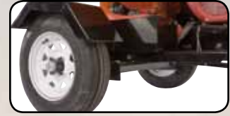
Large 12" tires/wheels and torsion axle makes this unit road-towable
